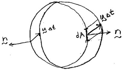
$$= \int_V \alpha_t dV + \lim_{\Delta t \rightarrow 0} \frac{1}{\Delta t} \int_{\partial V} \alpha(\underline{u} \cdot \underline{n}) dA$$
