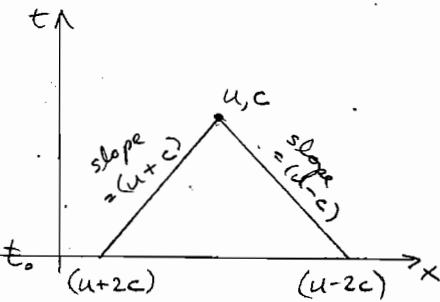
When there is no shock, for an infinitesimal time interval, there are two unknowns ( $u$  and  $c$ ) and two equations, one for each Riemann invariant:
